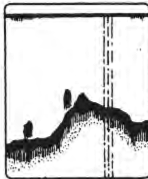
Interference from electrical equipment
