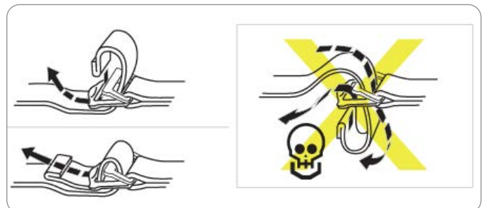
Correct threading of Deckvest 6D adjustment straps
