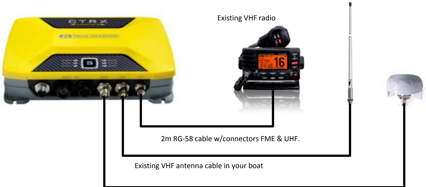
Cable, 5m, RG-58, attached to the GPS antenna
